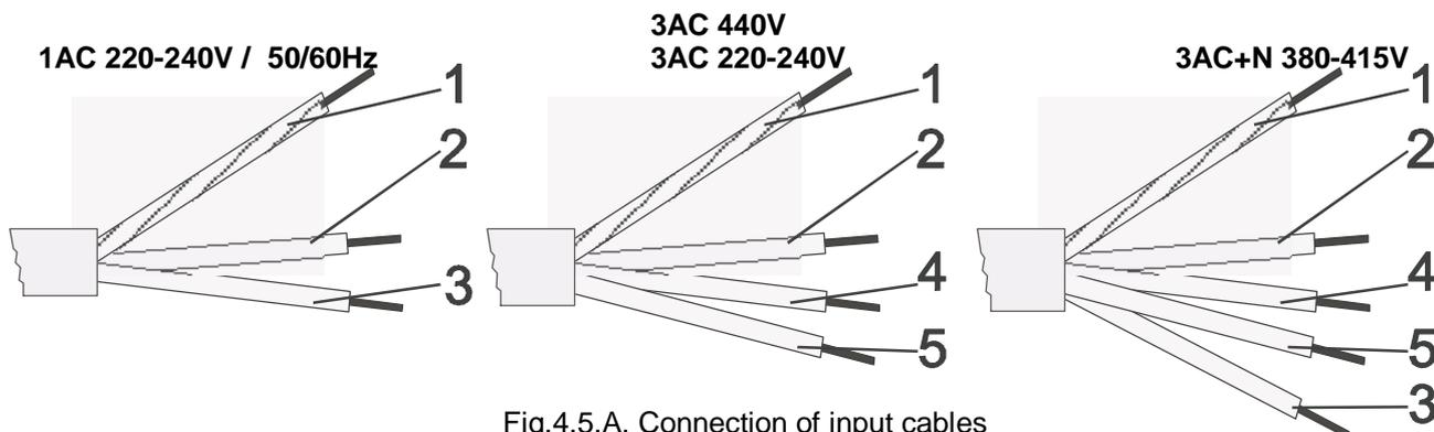
Fig.4.5.A. Connection of input cables
