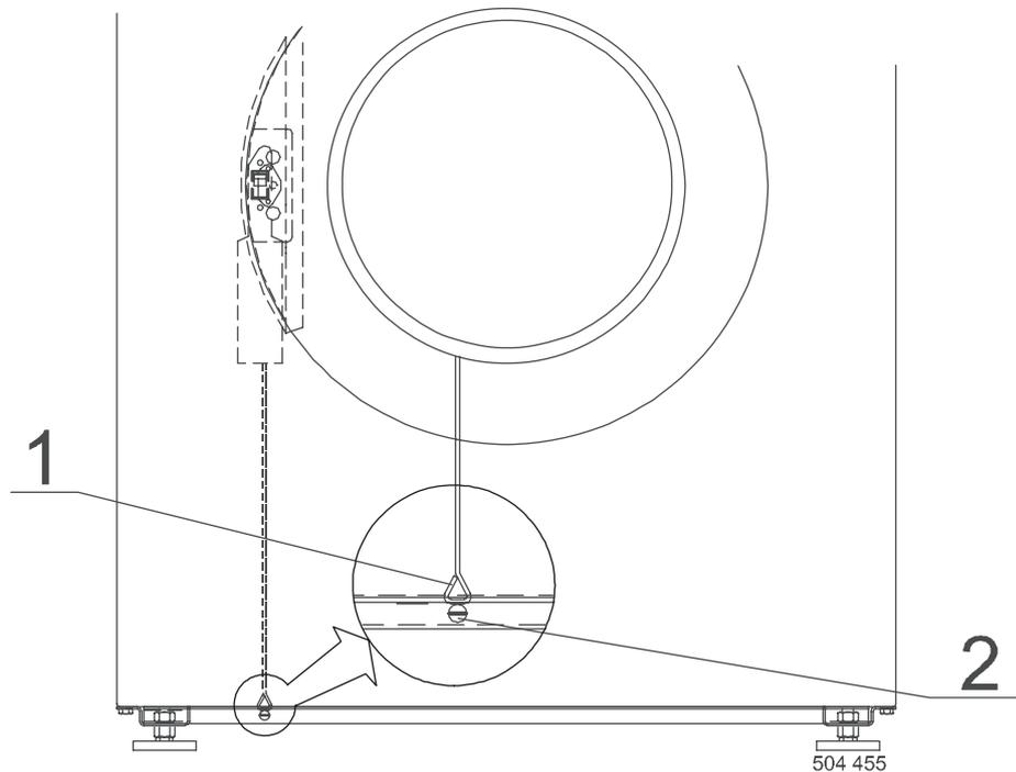
Fig. 6.1. Lever of emergency opening the door.
