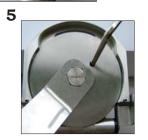
If the device is not used for longer periods, a more intensive cleaning is advisable. For this, unplug the device from the power supply as shown, dismantle the circular knife, loosen the knife head locking and remove the knife head. The device can now be cleaned. The device is assembled in the reverse order. Ensure that the knife head screw is not tightened too firmly and that the locking key is removed before operation!
